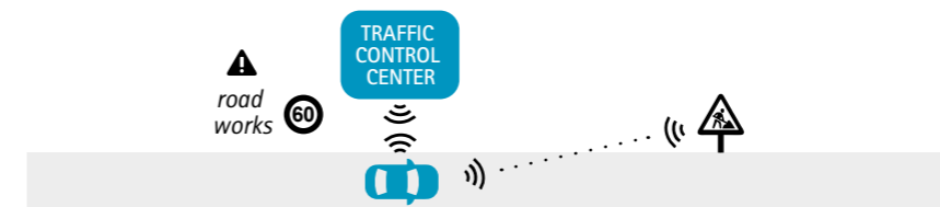
Figure 5: Road Works Warning: Drivers are informed about upcoming construction sites and their relevant data as well as any obstacles (e.g. closed lanes).
